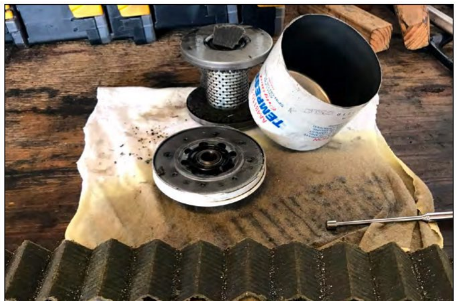
Fig. 1 Cutting open an oil filter
